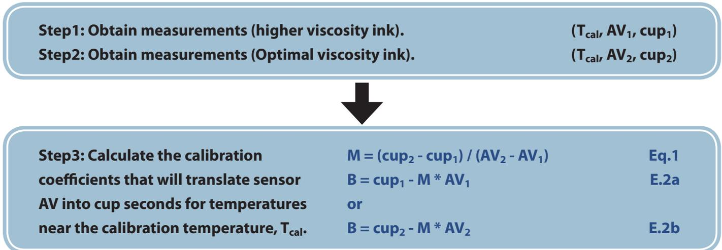
**Figure 1.** The calibration process flow diagram.
