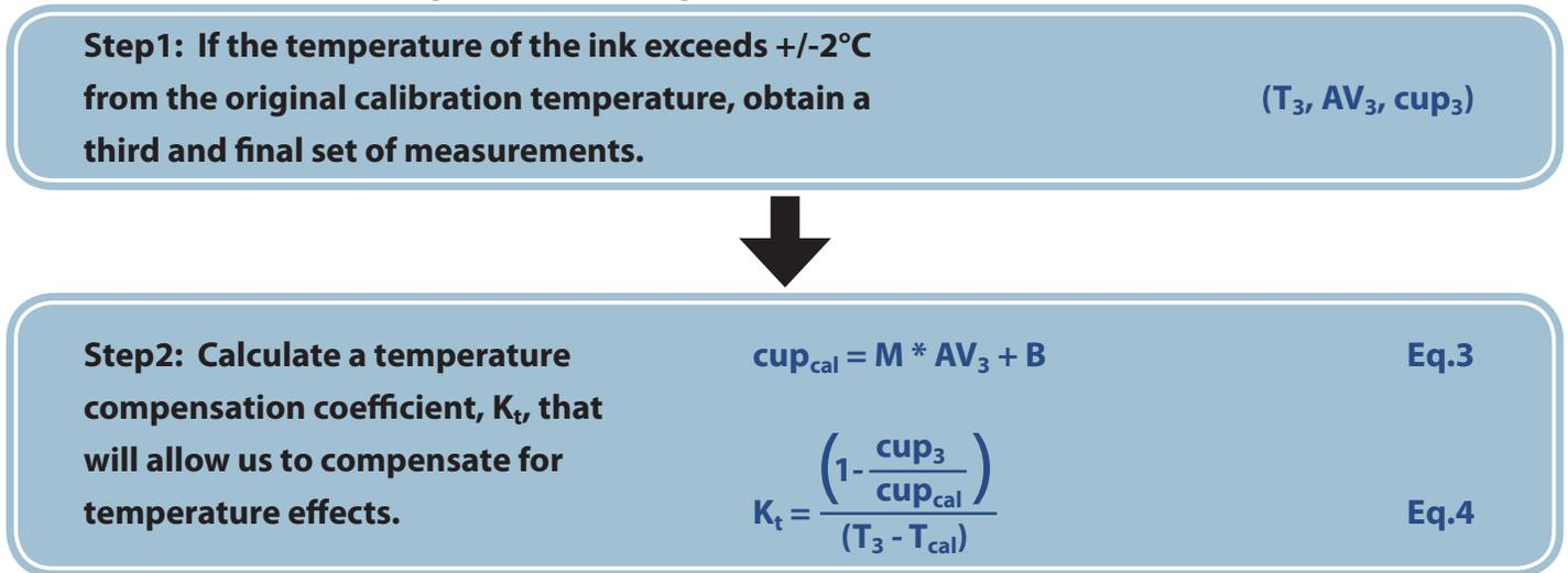
**Figure 2.**The secondary calibration process to compensate for temperature effects.
