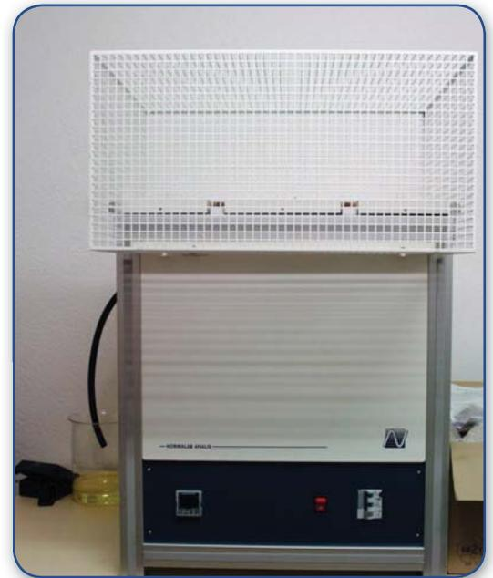
Figure 6a: Water bath for the RPVOT vessel.
