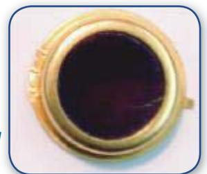
Figure 8: ViSmart™ sensor element at the conclusion of the RPVOT test showing full reliability and robustness
