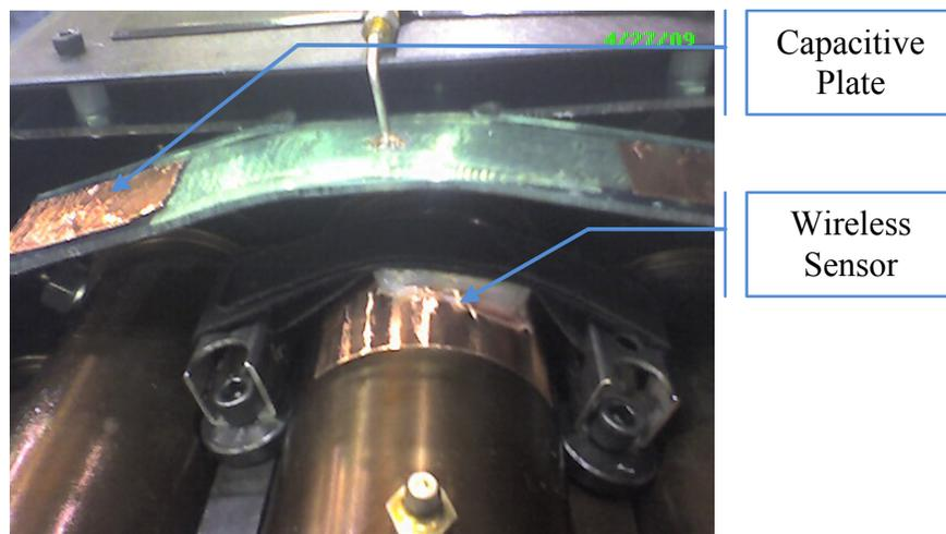
*Figure 3: Typical Installation on Rotating Machine Component*
