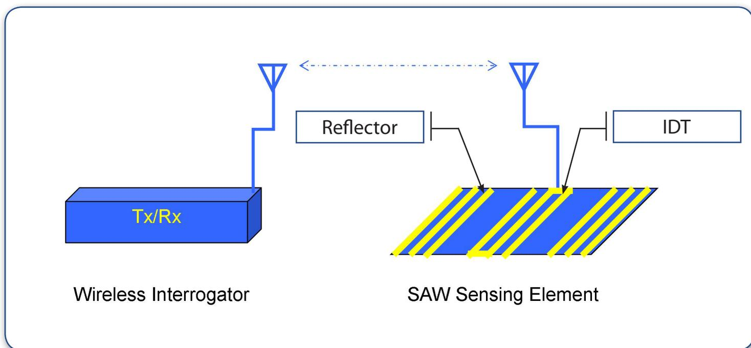
Figure 2: Wireless SAW Temperature Sensing System
