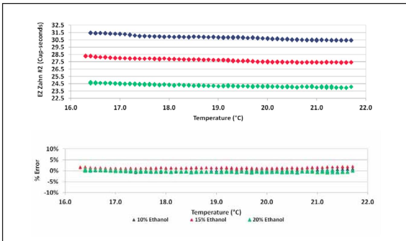
**Figure 4:** Calibrated sensor measurement vs. temperature for varied (10 percent to 20 percent) concentration of ethanol mixed into Flint CF white ink translated into EZ Zahn #2 cup-seconds and the associated error.
