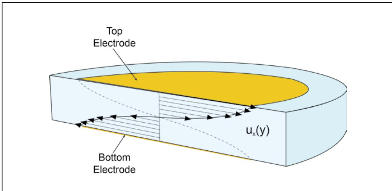
**Figure 1:** Increasing viscosity of a fluid placed on the top electrode results in an increase in the damping of the viscosity sensor and a decrease in the BAW's oscillator's frequency.
