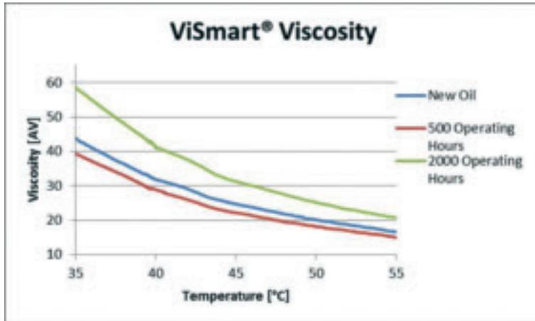
Fig.1. Viscosity change due to aging.
