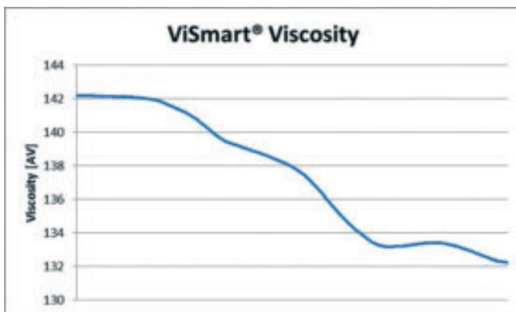
Fig.2. Viscosity change due to contamination (ISO VG46 with VG32).
