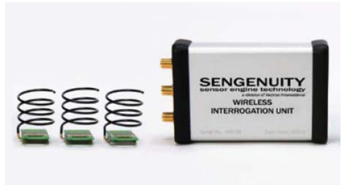
Figure 5. The interrogation unit (reader) and three typical SAW temperature sensor modules. The sensor elements are 3.8mm x 3.8mm ceramic-packaged resonators embedded in the PCB package. The coil antenna shown has been designed for operation in the vicinity of 433 MHz with a desirable radiation pattern.
