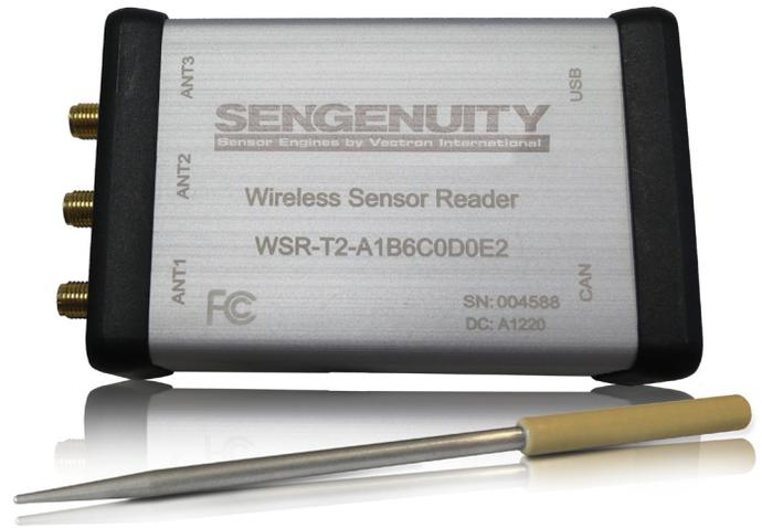
Figure 1: Food Probe with Wireless SAW Reader
