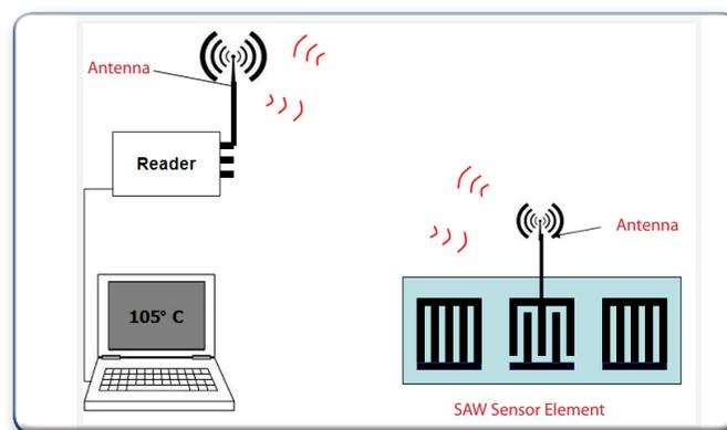
Figure 2: Wireless SAW Temperature Sensing System
